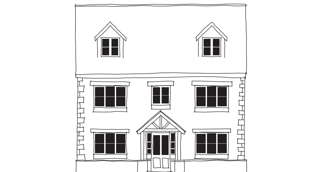
2.5 storey dwelling with pitched dormers, stone headers and cills and dressed stone quoins
