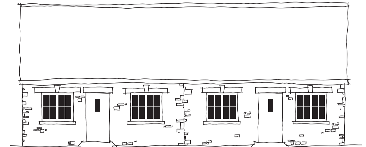
Bungalows in rubblestone with stone headers and cills
