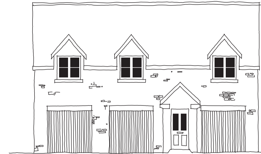
Flat over garage (FOG) with dropped eaves and gablets for mews streets
