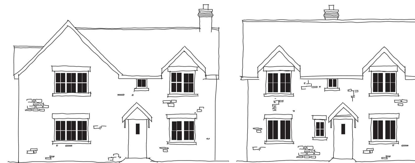
Front Elevation Side Elevation Pair of 3 bed dwellings arranged to turn a corner with prominent gables and pitched door canopies
