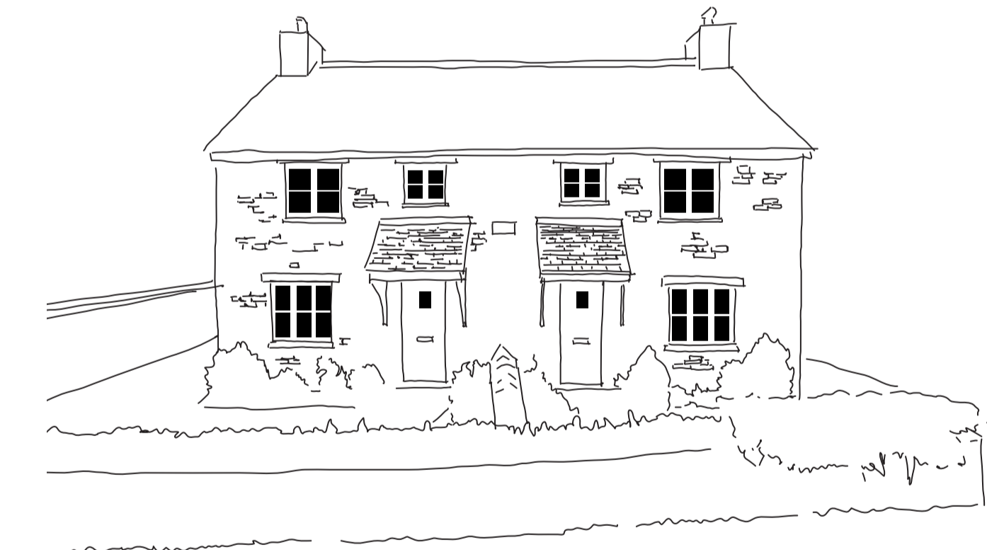
Terrace of smaller dwelling types in rubblestone with pitched porches and stone detailing
