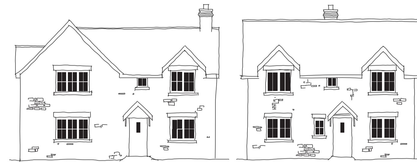
Front Elevation Side Elevation Pair of 3 bed dwellings built in stone and arranged to turn a corner with prominent gables and pitched door canopies.
