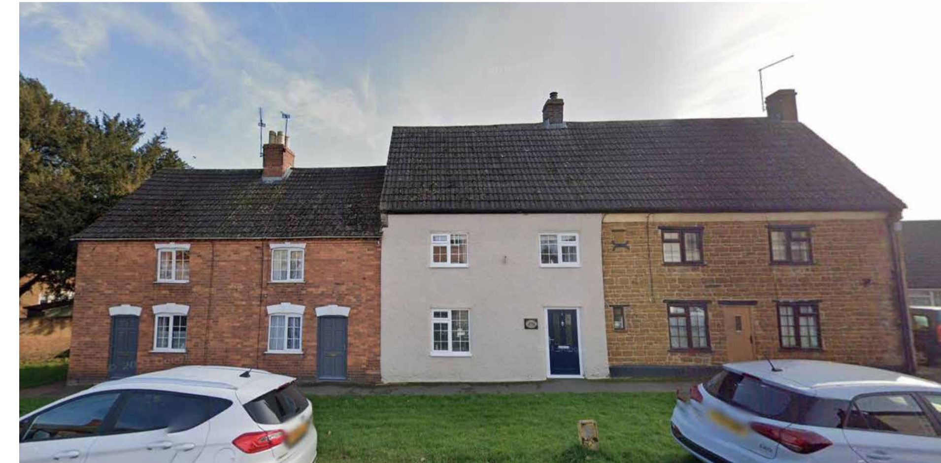
High Street - The typical mix of building materials within Braunston includes red brick in various tones and textures, limestone, Ironstone, cement render in off-white shades, Welsh slate, Collyweston stone slate and roof tiles (mixed grey and red types).
